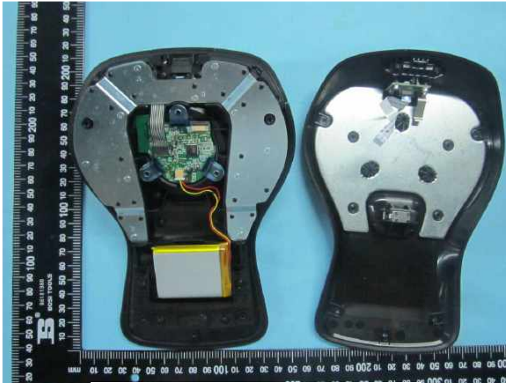
Space Mouse Pro Wireless Cover Off - Front View
